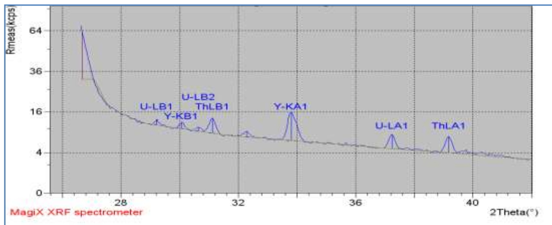
Figure1.Detectionof uraniumpeak usingthecrysta lLiF220
