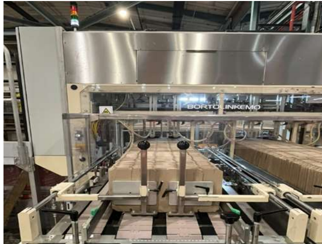
Figure 2. Div-Inserter and associated packaging machinery
