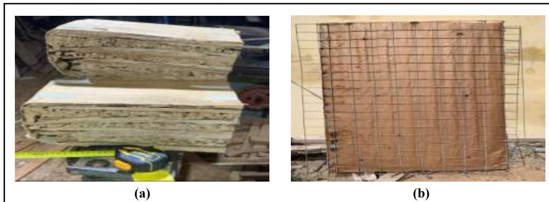
Figure 1. Samples of typha chipboard panels seen in profile (a) and from the front (b)
