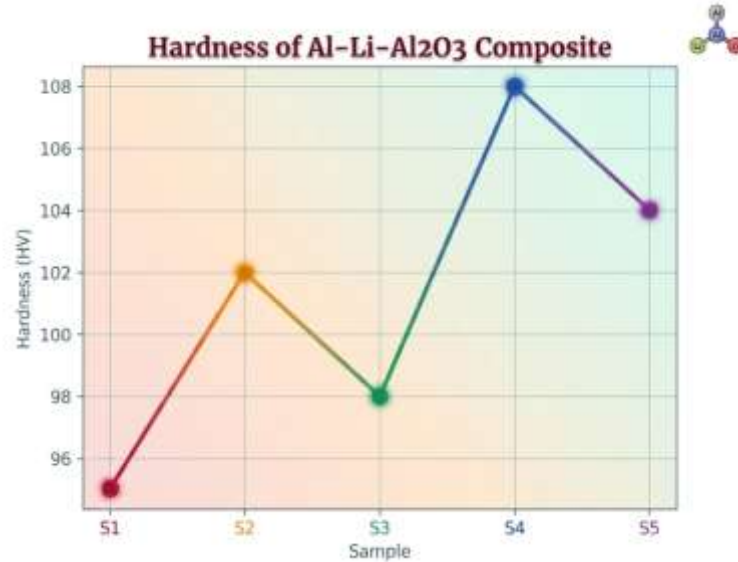
Fig 2 ;Hardness testing graph of Al-Li-Al 2 O 3 composite
