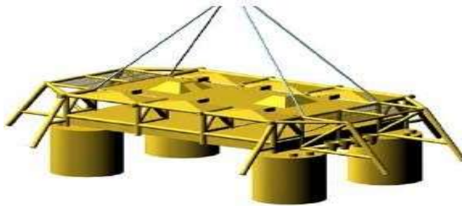
Figure 4. A subsea template
