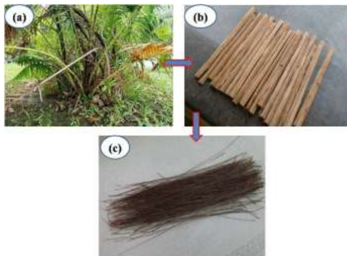
Figure 1. (a) Rattan plant, (b) stem and (c) extracted fibers from RA stem.
