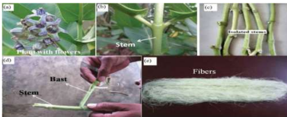
Figure 1. Calotropis gigantea (a) plant (b) stem (c) extracted stem (d) extracted bast from stem (e) extracted fibers.
