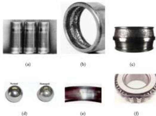
Figure 5. (a) Wear of rolling elements (b) Corrosion of the outer ring (c) Friction of the rolling surface (Hamouche, 2022) (d) Defect on a ball (e) Spalling of the inner ring (e) Spalling of the outer ring (f) Deformation of the cage (HOTAIT, 2020)
