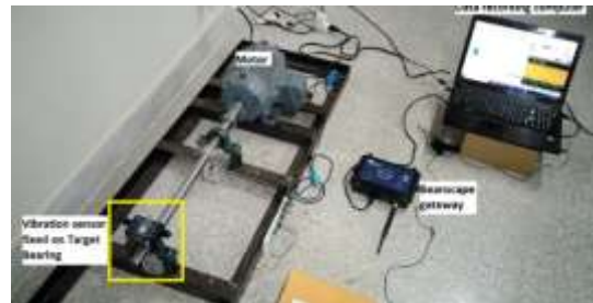
Figure 3. Test bench used by Aziz & al. (2023) for acquiring vibration signals from bearings. The mechanical device includes an electric motor, frame, bearings and shaft simulating different operating states: normal operation, inner ring defect and outer ring defect
