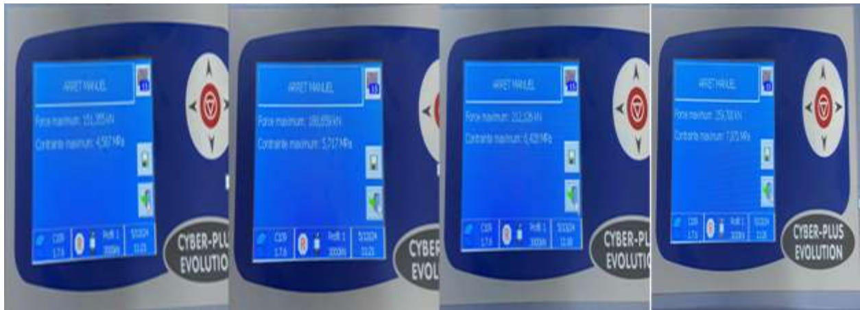
Figure 8: Stresses and fracture loads of the specimens
