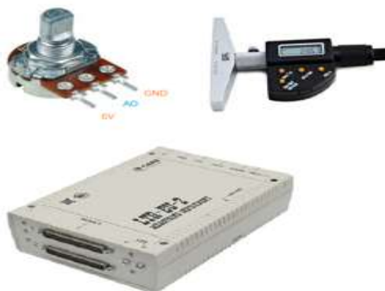
Fig. 6. Potentiometer, depth gauge GMC-100 0.001 electric, LTR-EU-2 crate with LTR212 module
