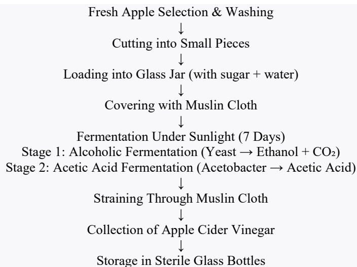
Flow Chart — Preparation of Apple Cider Vinegar from Apple Pulp:
