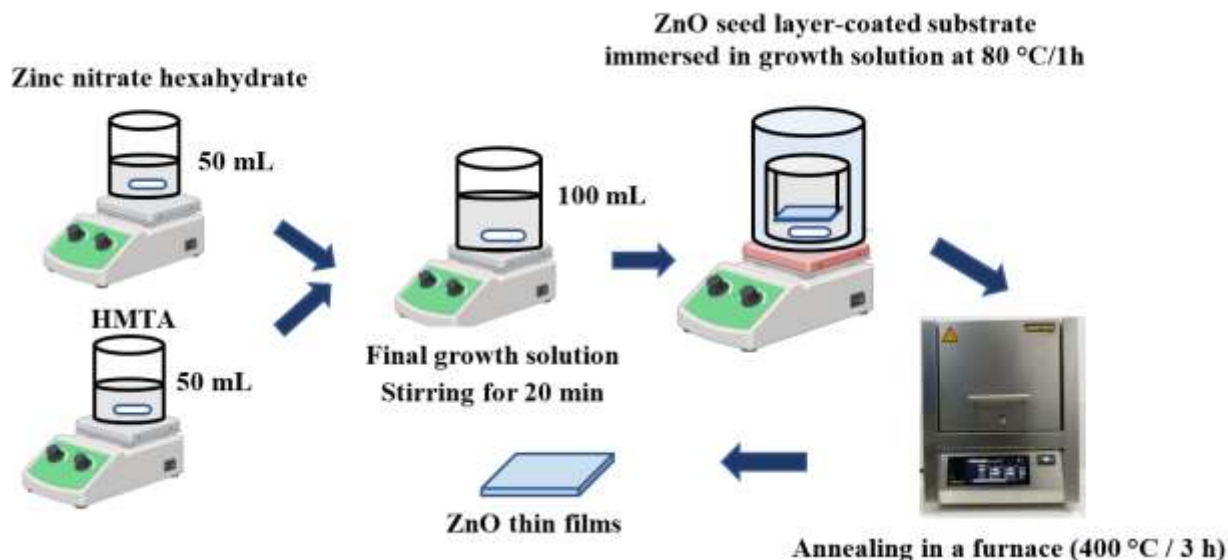
Figure 2: Schematic illustration of the ZnO thin films deposition process by chemical bath deposition (CBD).
