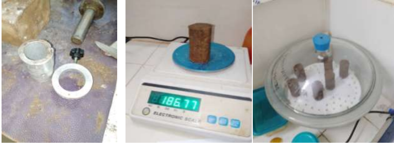
Figure 6. Specimen preparation steps(specimens 38 mm in diameter and 76 mm in height).
