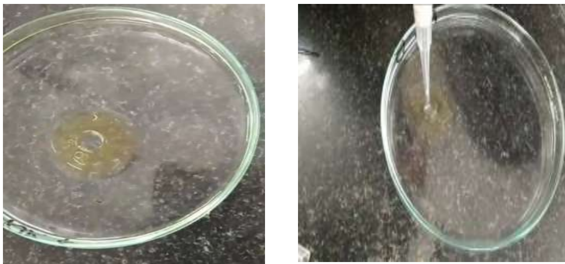
Fig 3 Foam Forming Activity of bacterial biosurfactant
