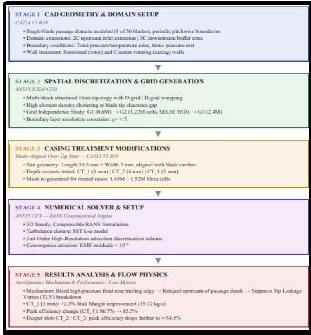
Figure17. Stages of CFD Methodologies used in Research
