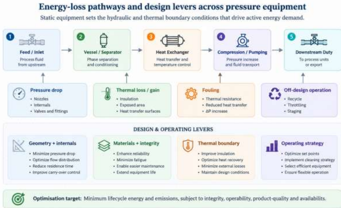
Figure 1. Energy-loss pathways and design levers linking pressure equipment to plant energy demand.
