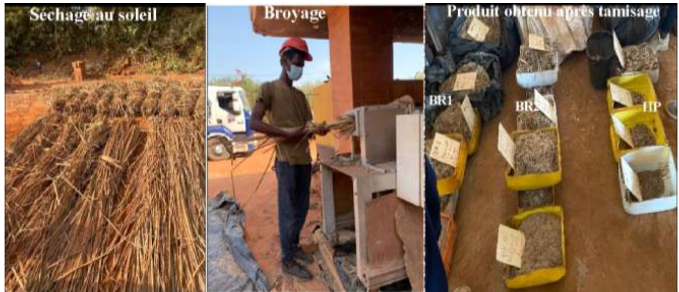
Figure 4:-Product after crushing Typha according to three methods
