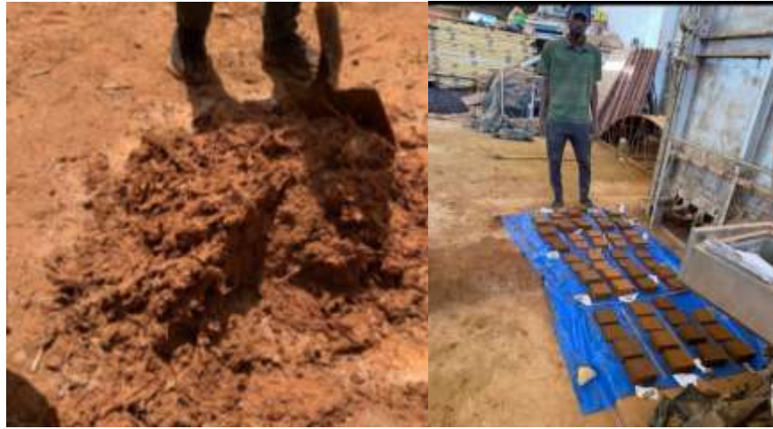
Figure 5:-Typha-based adobe bricks
