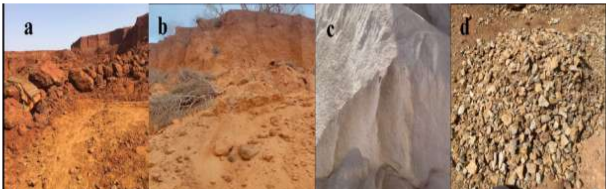
Figure 2:-The raw materials to be used for the formulation of laterite adobes: Sindia (a), keur mori sand (b), Bandia limestone (c) and thicky clay (d)
