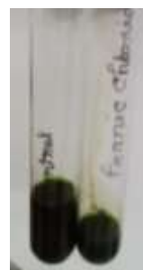
Figure 3.14: Ferric Chloride Test
