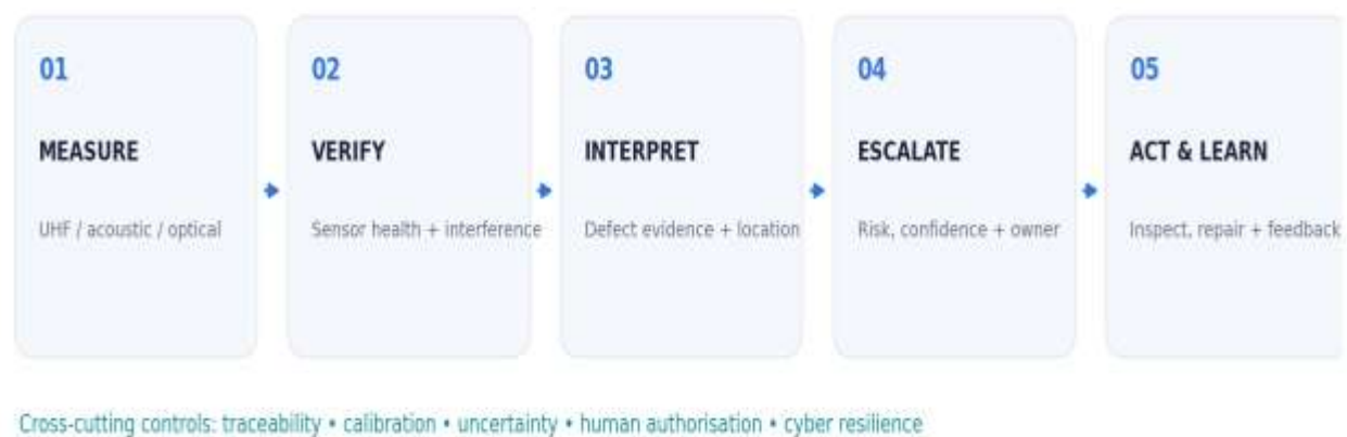
Figure 1. Proposed quality-controlled signal-to-action workflow for an operating GIS asset (author synthesis).
