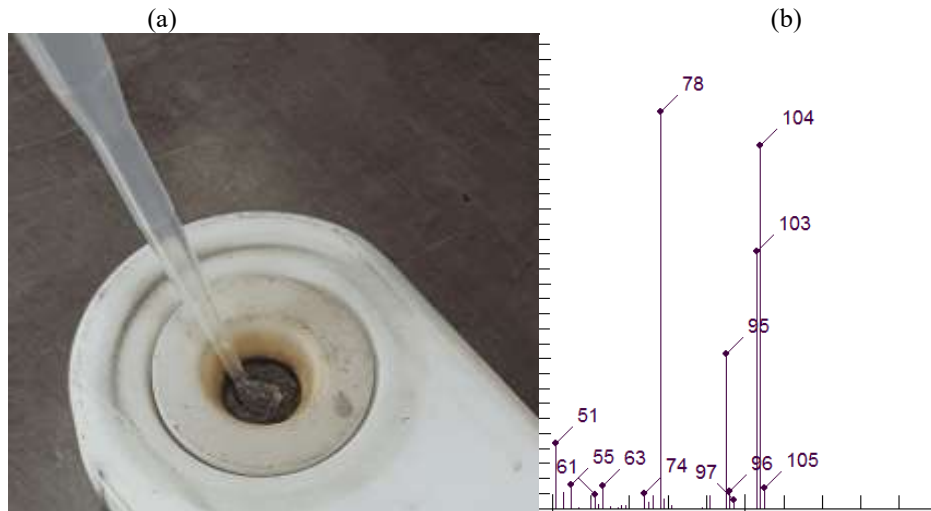
Figure 5. Test 1: (a) direct application of the PSL-simulant mixture to the filter and (b) the resulting mass spectrum.
