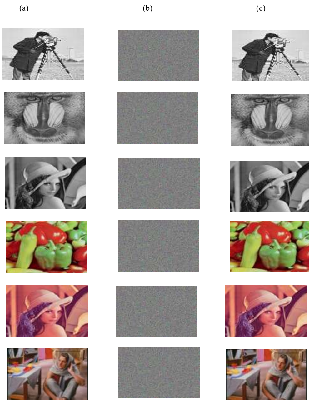
Fig 4. Visual evaluation of the proposed HCES image encryption and decryption scheme. (a) Original plaintext images; (b) corresponding encrypted ciphertext images exhibiting noise-like visual patterns; (c) decrypted images recovered using the proposed decryption procedure.
