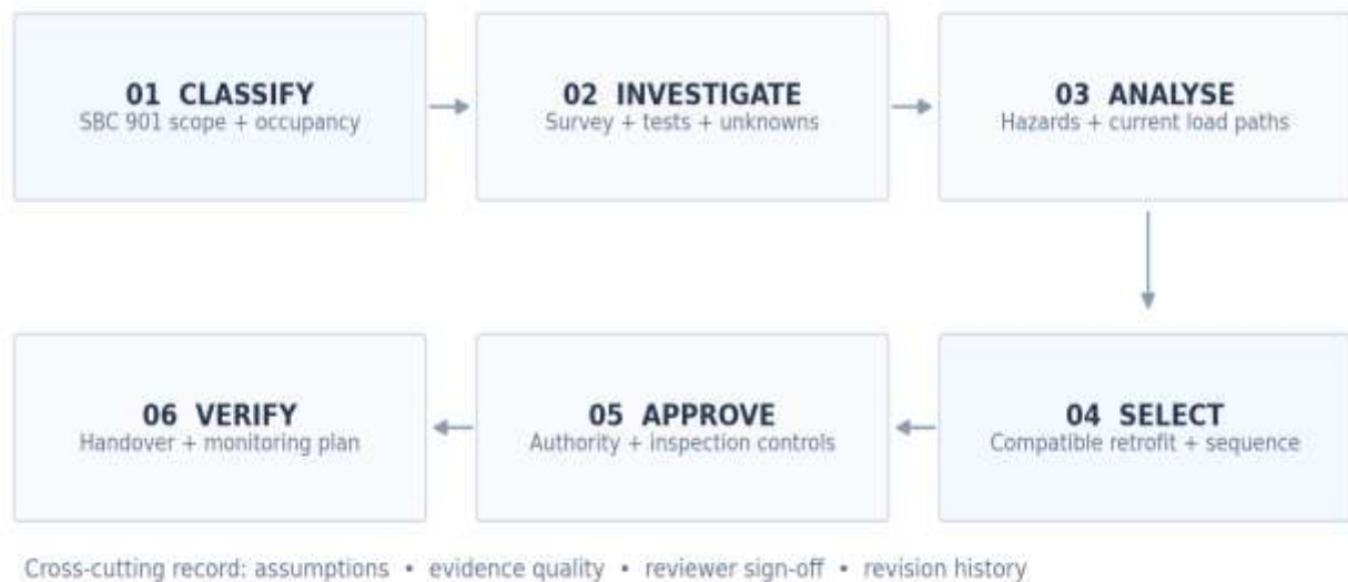
Figure 1. Proposed six-stage code-oriented evidence and approval sequence (original schematic).
