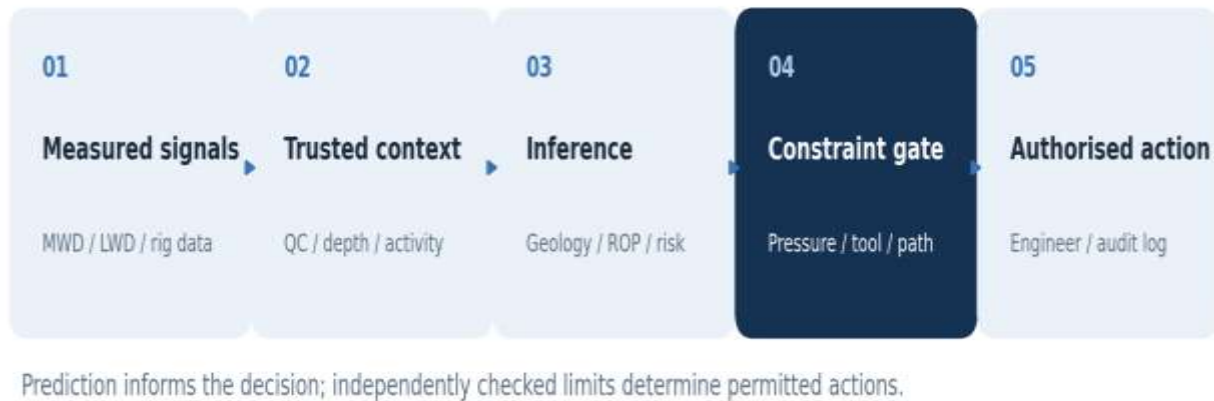
Figure 1. Proposed sensing-to-authorisation architecture for supervised drilling optimisation.
