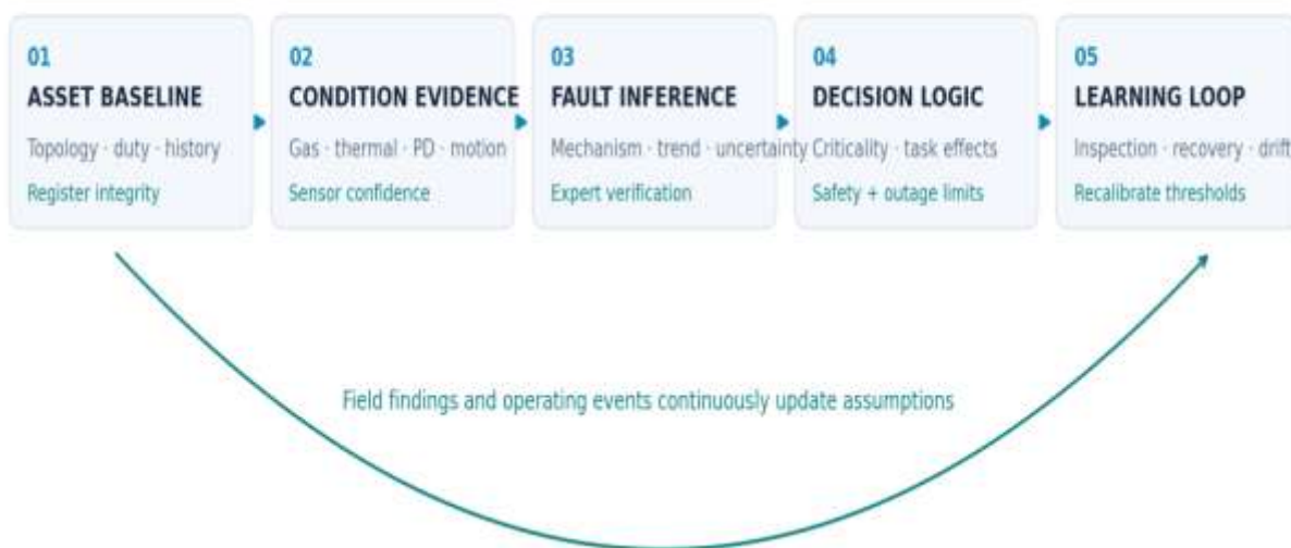
Figure 1. Proposed condition-to-decision architecture for industrial electrical assets. Original conceptual figure.
