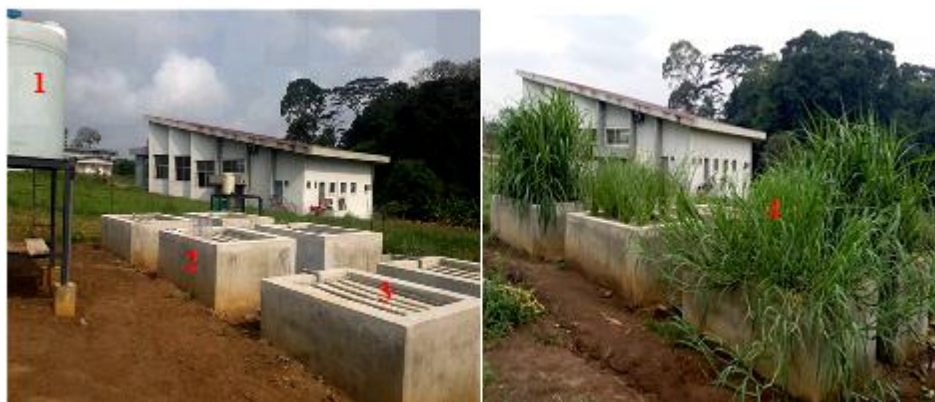
Fig.1:- View of the experimental wetland system, 1: feeding tank, 2: bed, 3: Irrigation device and 4: plants growing on the beds after two months.
