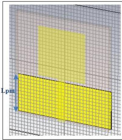
**Fig 7:-** Reducing the length L<sub>pm</sub> of planar microstrip antenna ground plane
