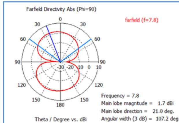
**Fig. 16;-** Two-dimensional radiation diagram of the ULB planar antenna at the 7.8 Ghz frequency in E plane (variable theta and constant phi).
