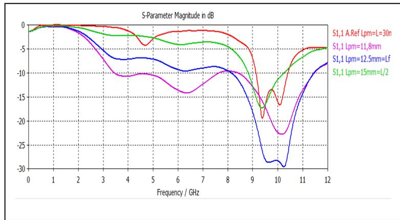
**Fig 8:-** Return loss S<sub>11</sub> versus frequency After Reducing the length L<sub>pm</sub> of planar microstrip antenna ground plane
