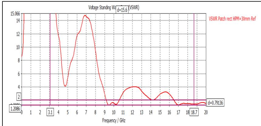
Fig. 13:- Standing Wave Ration SWR versus frequency for starting antenna with total ground plan dimensions 30x30 mm<sup>2</sup>
