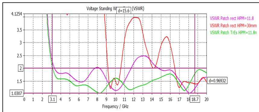
Fig. 14:- Standing Wave Ration SWR versus frequency for three antennas : starting antenna, without and with gradual transition between planar patch and microstrip feed line.
