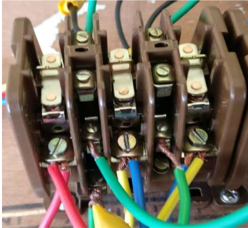
Figure 4.1:- Contactor: 18A 230 VAC ratings
