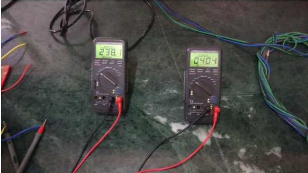
Figure 3.4:- Readings of line voltage and phase voltage for 3 phase star (starting condition)
