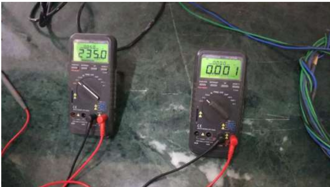
Figure 3.5:- Readings for line voltage and phase voltage for 3 phase Delta position (running condition)
