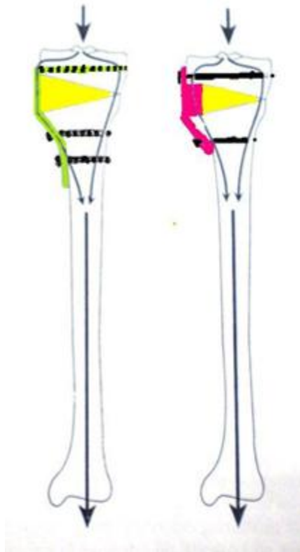
Figure 1. Axial forces exerting shear stress on the plate without step at the site of opening wedge leading to loading of screws and with the step at the site of opening wedge preventing loading of screws and transmitting axial force in a direct line.
