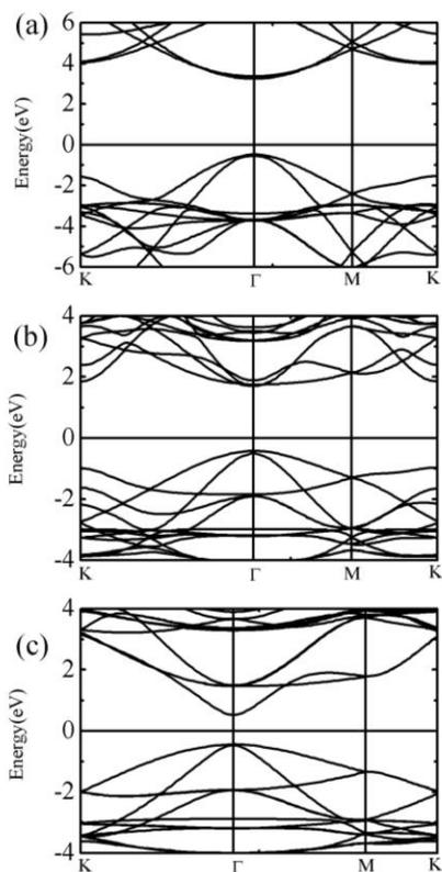
**Fig-3.** The band structures for Fully hydrogenated group-IV nanosheets. (a) for graphene; (b) for silicene; (c) for germanene.
