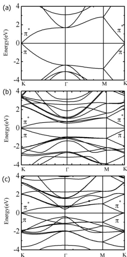
**Fig-1.** The band structures for pristine group-IV nanosheets. (a) for graphene; (b) for silicene (c) for germanene.
