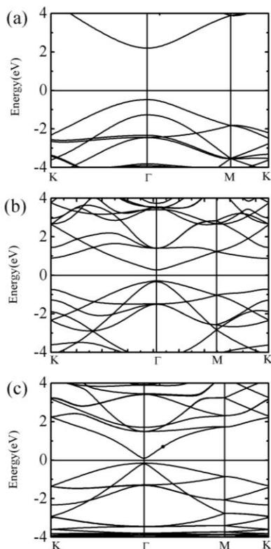
**Fig-4.** The band structures for Fully fluorinated group-IV nanosheets. (a) for graphene (b) for silicene (c) for germanene.
