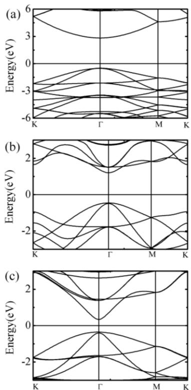
**Fig-5.** The band structures for Group-IV nanosheets codoped with H and F. (a) for graphene (b) for silicene (c) for germanene.
