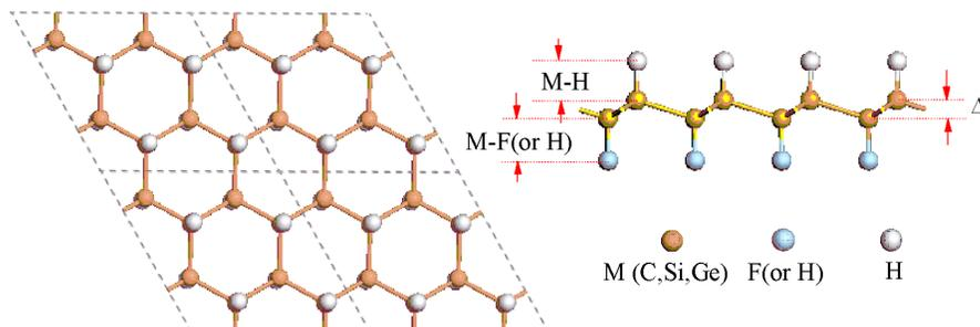
**Fig-2.** The schematic diagram of group-IV nanosheets decorated with H and F atoms. Left panel and right panel represents top view and side view. Purple spheres are group-IV (C, Si, Ge) atoms, white for H atoms, and blue for F atom but also stand for F atoms when system fully hydrogenated.
