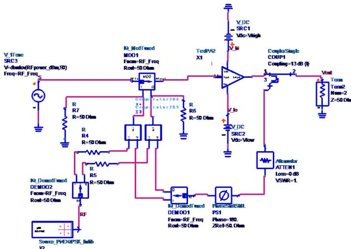
Fig.8 closed loop Cartesian feedback
