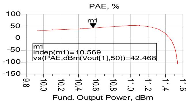
Fig. 5: PAE of the designed PA
