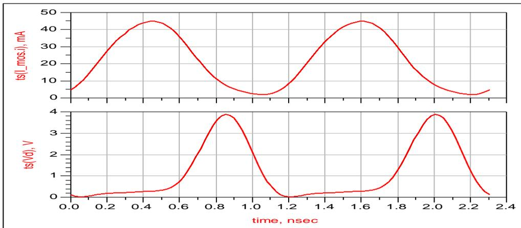
Fig.4 voltage and current waveform at the drain of the MOS Transistors
