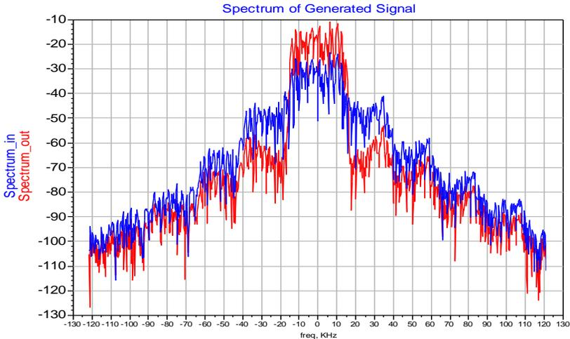
**Fig.9-b** linearized P.A. spectrum
