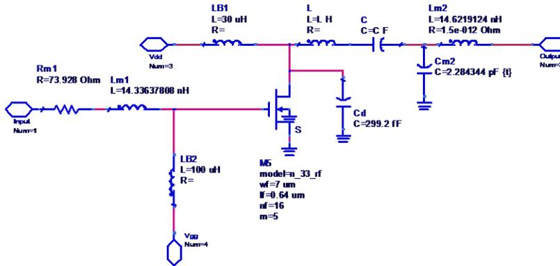
**Fig. 2 Zigbee class E Power Amplifier**
