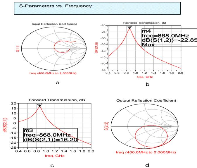
**Fig.3.a**  $S_{1,1}$  matching, **Fig.3.b**  $S_{2, 2}$  output matching, **Fig.3.c.** reverse transmission, **Fig.3.d** Forward Transmission
