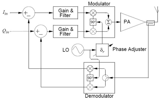
Fig. 1: Cartesian feedback transmitter.
