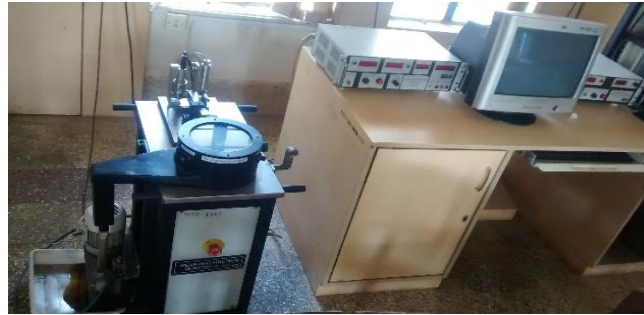
Fig. 4. Experimental Pin on Disc Lab Set Up
