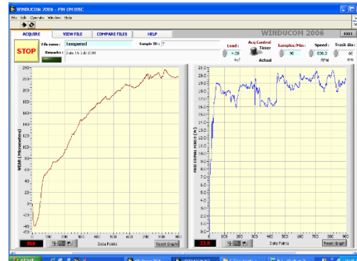
Fig 6. Wear & Frictional Force graph for Tempered Specimen at 4 Kg.
