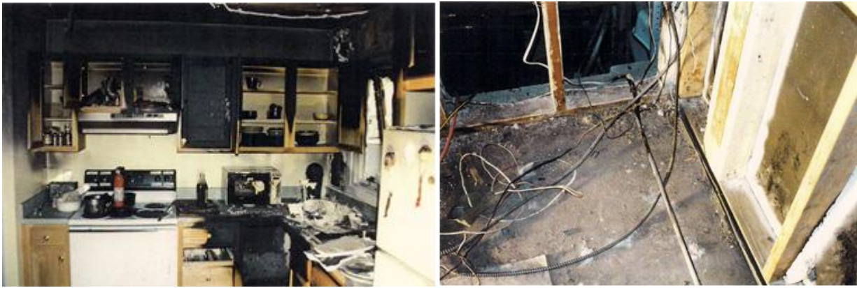
Fig. 1: (a) The kitchen after the fire. Fire extinguisher on top of stove is un-used. (b) Fridge wire (long straight wire) was found as the point of ignition for the kitchen fire.
