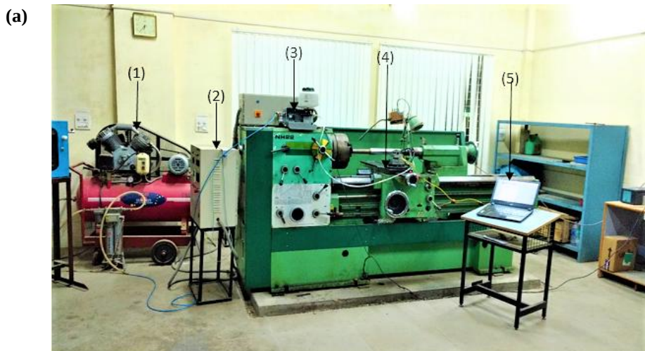
(1) Air Compressor (2) Control Panel (3) MQL Setup (4) High-speed precision lathe machine (5) PC attached with thermocouple
