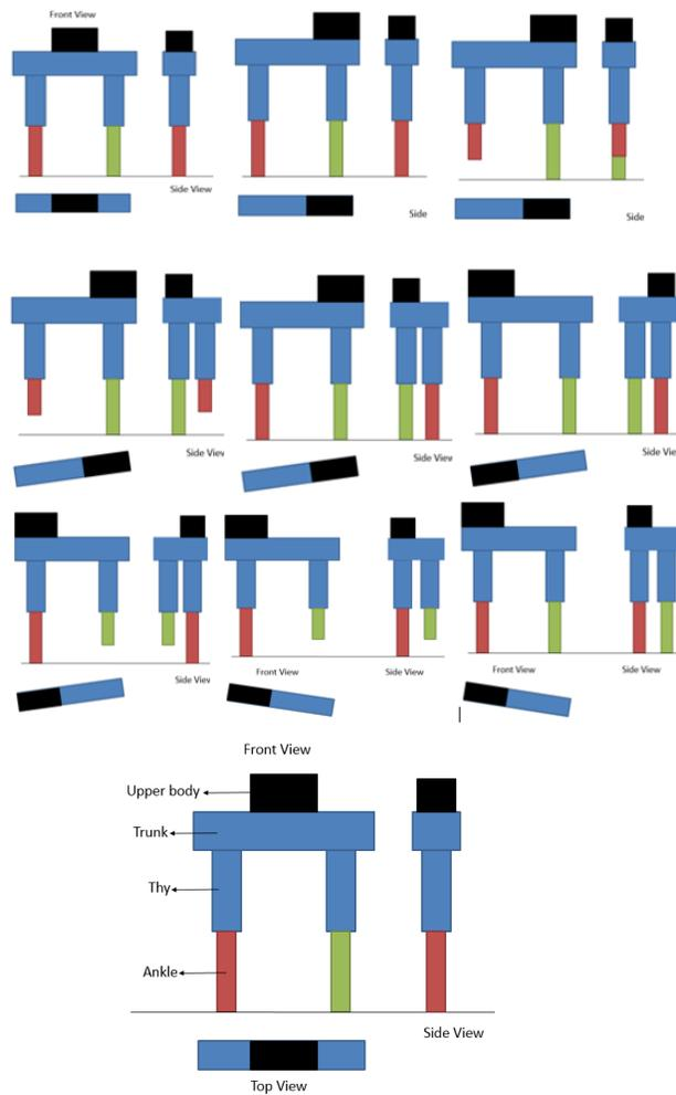
Fig 3.2 Figure of walking gait of the robot
