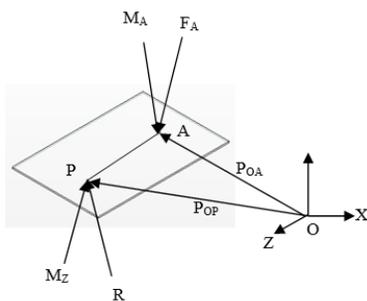
Fig 3.2 Forces acting on the robot ZMP
