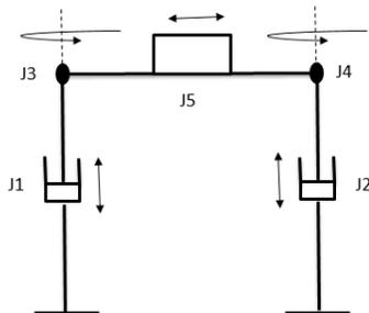
Fig 2.2 Figure showing different joints of the walking robot
