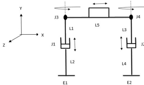
Fig 3.1 Figure of forward kinematics of the robot
