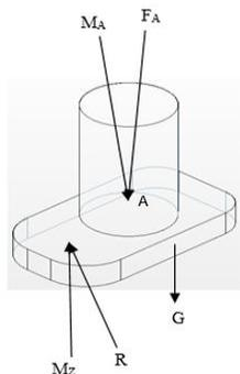
Fig 3.4 Zero moment point of the robot foot
