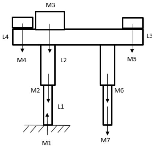
Fig 3.6 Torque at hip of the walking robot
