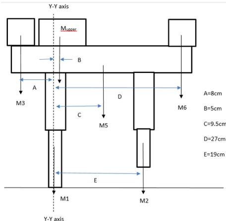
Fig 3.5 Mass distribution of the walking robot
