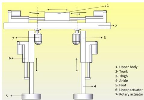
Fig 2.1 CAD model of the walking robot showing the parts of the robot
