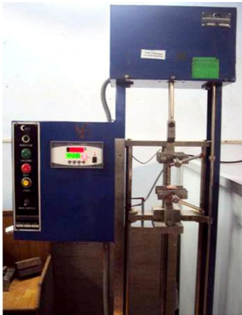
Figure 2: universal testing machine for testing the pull out bond strength.
