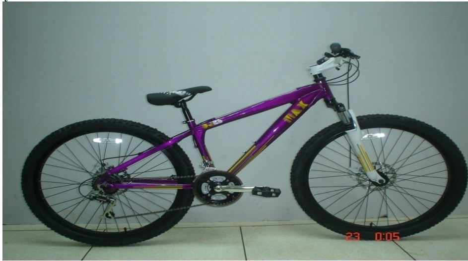
Fig-1:- Max 26 inch 18 speed Racing Bicycle.
