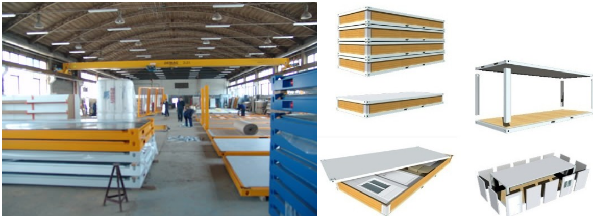
Figure 5:- Assembled and disassembled form of prefabricated modular container,
