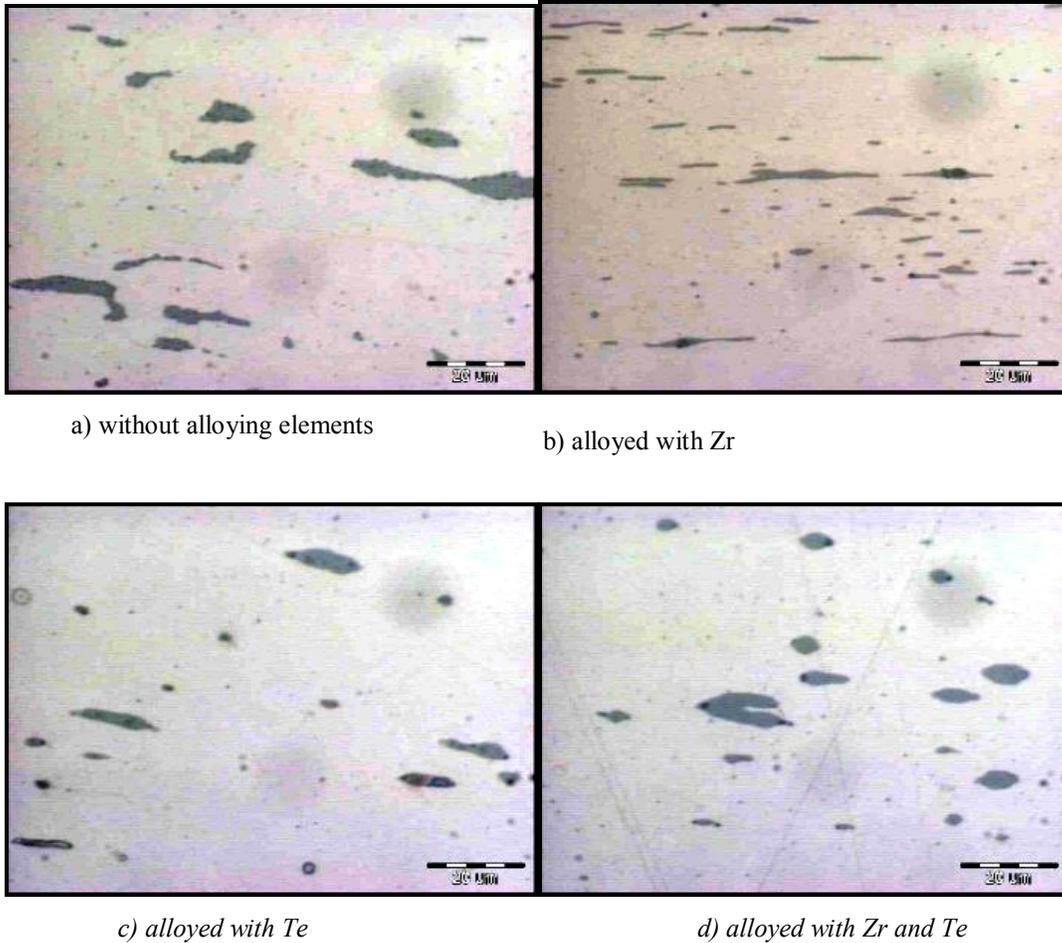
**Figure 8:-** Microstructure of all melt variants for rolled state [9].
