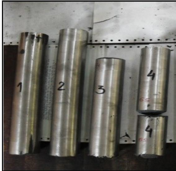
Figure 5:- The samples after the completion of forging process and rough machining [9].
