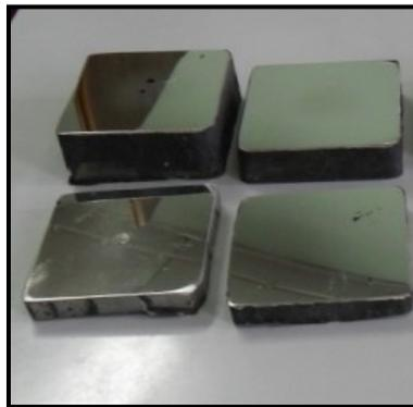
Figure 3:- Casted samples for metallographic tests [9].
