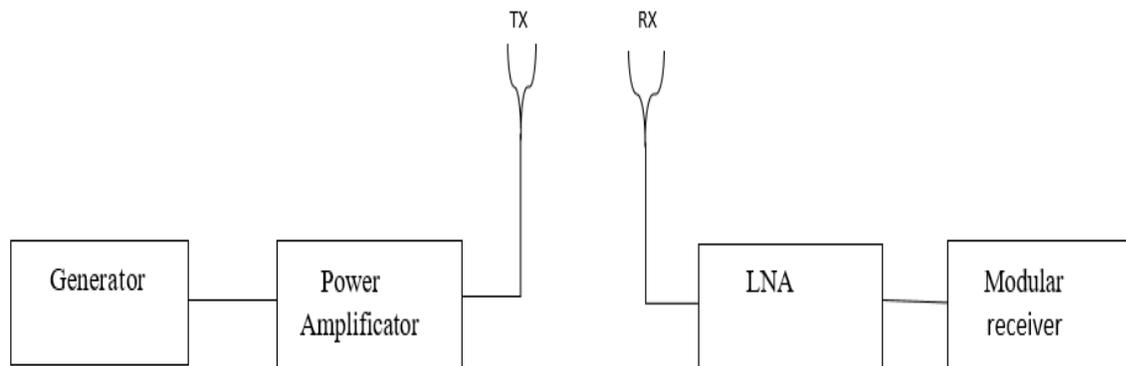
Figure 3:- Simplified transmission chain.
