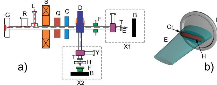
Figure 1.a) Experimental setup of AREAL facility, b) beam-sample overlapping. G – Electron gun, R – RF input, L – Laser beam, S – Solenoid magnet, C – Corrector magnet, D – Dipole magnet/spectrometer, Y – YAG screen, T – Titanium window, E – Electron beam, B – Beam dump, H – Sample holder, F – Faraday cup, X1, X2 – Experimental stations, Cr – beam cross-section.
