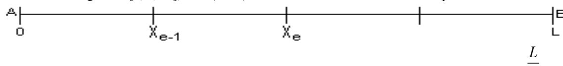
Figure 1:- One dimension domain divided into four elements mesh size= $h_e = \frac{L}{4}$
