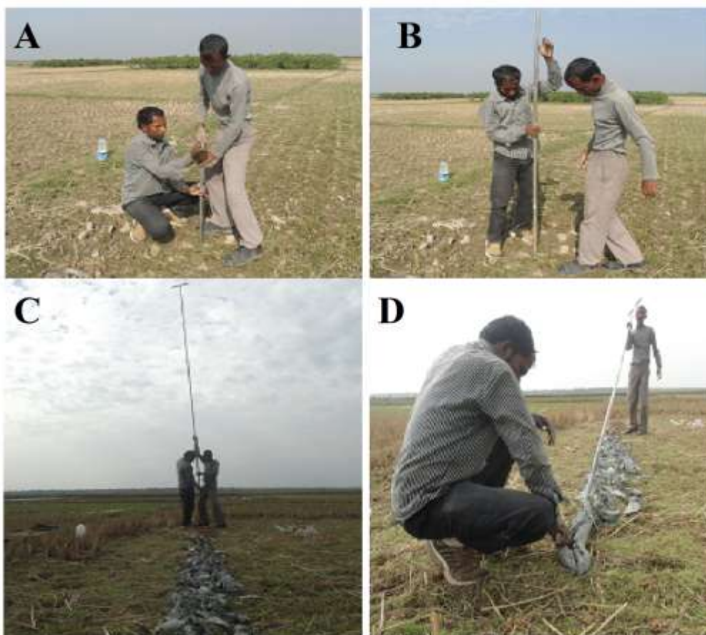
Plate-1:- The white clay exploration activities using auger method/shallow boring method; (A) An auger is vertically penetrating the subsurface, (B) A close view of auger removing from the hole, (C) Whole auger view after removed from the hole, (D) Finally, the sample was cutting and laid in a line to maintain consistency of operation, Madhabpur area, Habigonj district.
