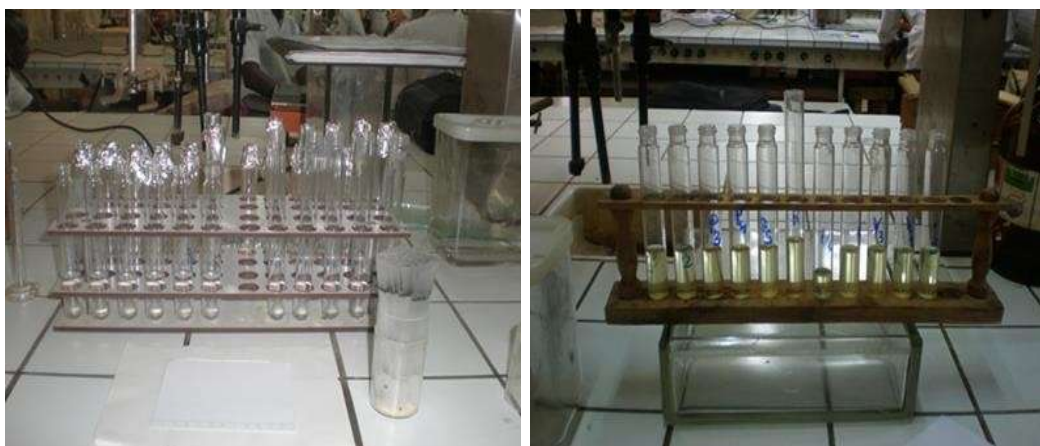
Figure2:- Weighing and solutions of the different samples in test tubes ready for TLC spotage.
