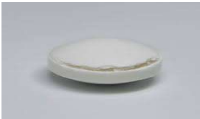
Figure2:- Delamination of bilayer tablet
