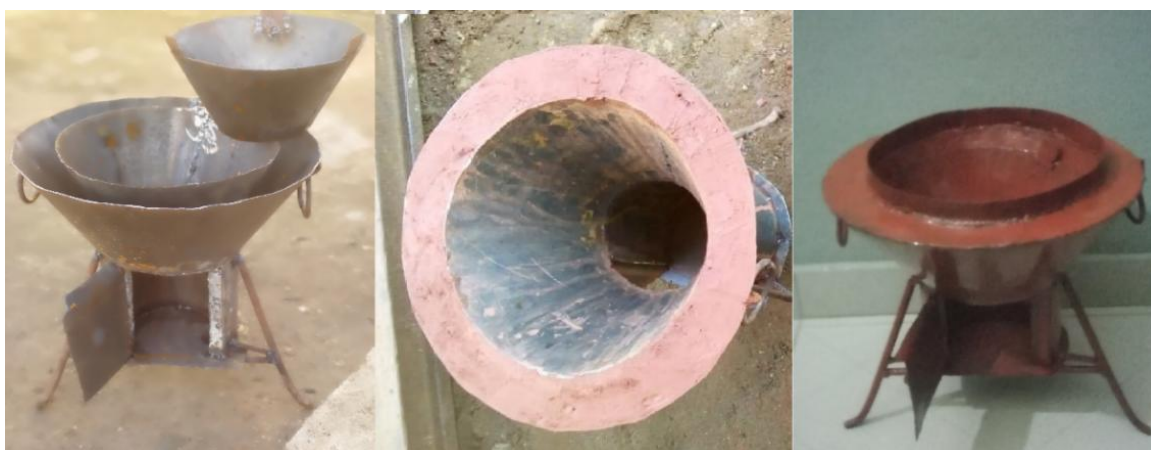
Figure 1 a:- Steps in designing of the conical cooking stove incorporating clay.
