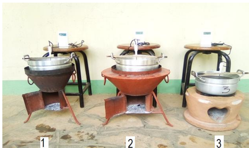
Figure 1 b:- Cookestoves tested: 1-Conical cookestove, 2- Modified conical cookestove, 3 clay cookestove.
