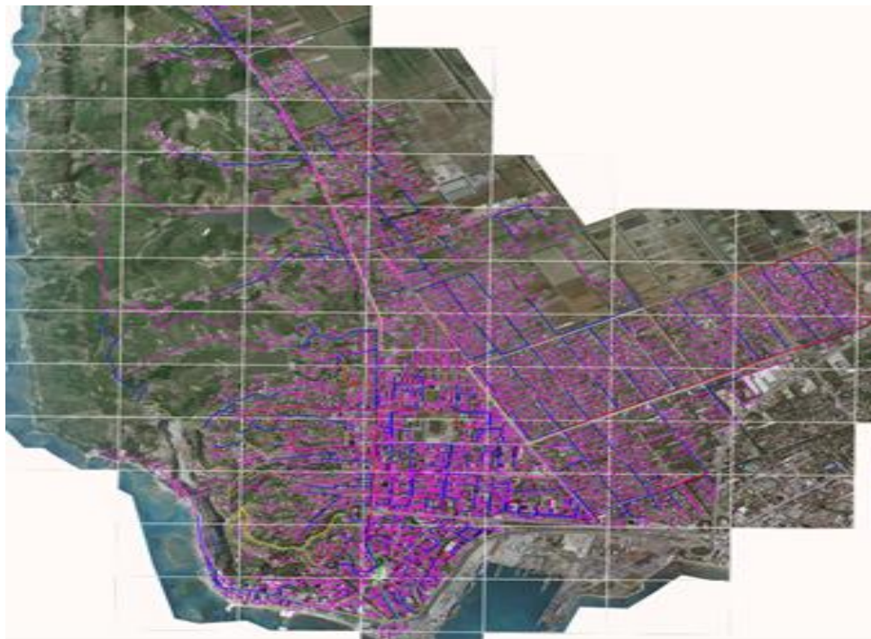
Fig.7:- Water distribution network.
