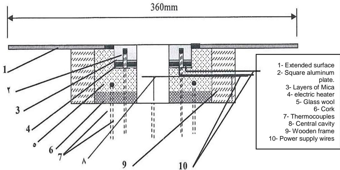
Figure (3):- A cross section showing the thermal insulation process.
