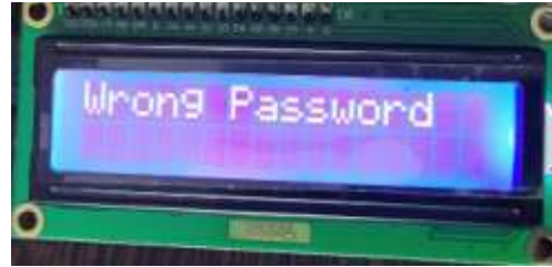
Fig.5:- LCD display as invalid password.
