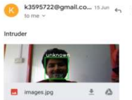
Fig.11:- Face Recognition output when not matched with the database.
