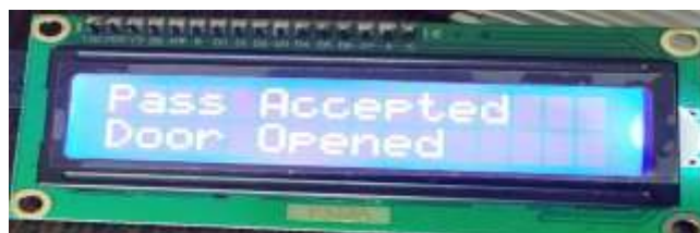
Fig.4:- LCD display as pass accepted.
