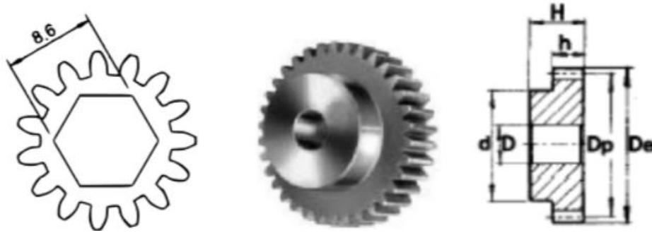
Figure 3:-Gear specifications.
