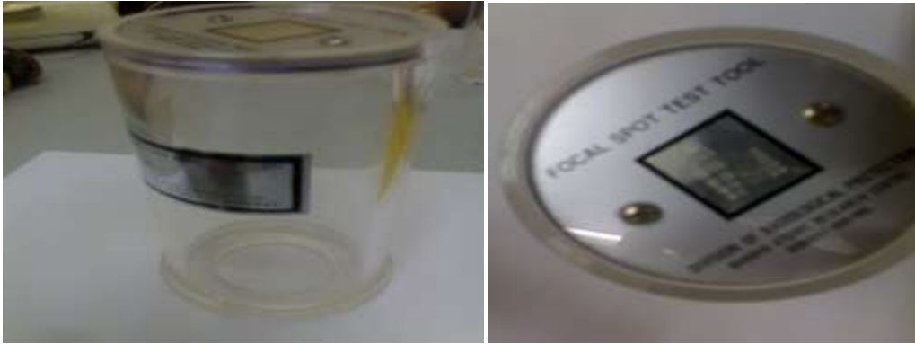
Fig 4:- Focal spot test tool with non-screen film cassette.
